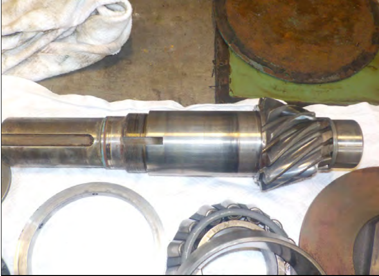
INPUT SHAFT AND BEVEL PINION (12T)
