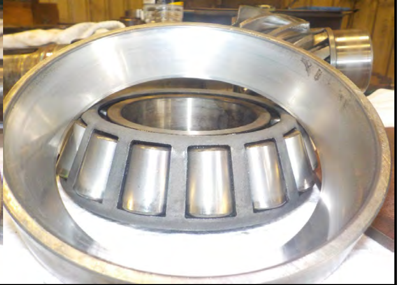
INPUT TAPERED ROLLER BEARING
