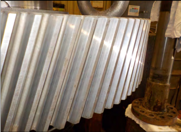
L.S. GEAR (113T) POLISHING
