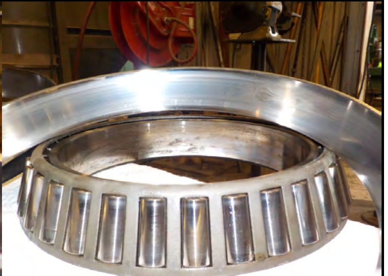
OUTPUT SHAFT TAPERED ROLLER BEARING
