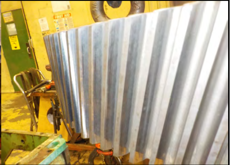
L.S. GEAR (113T) POLISHING
