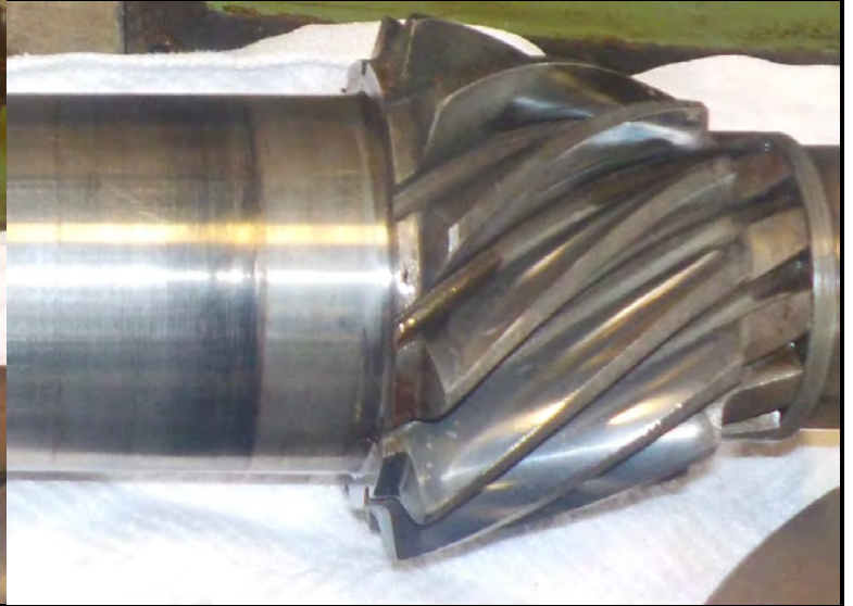
BEVEL PINION (12T) POLISHING
