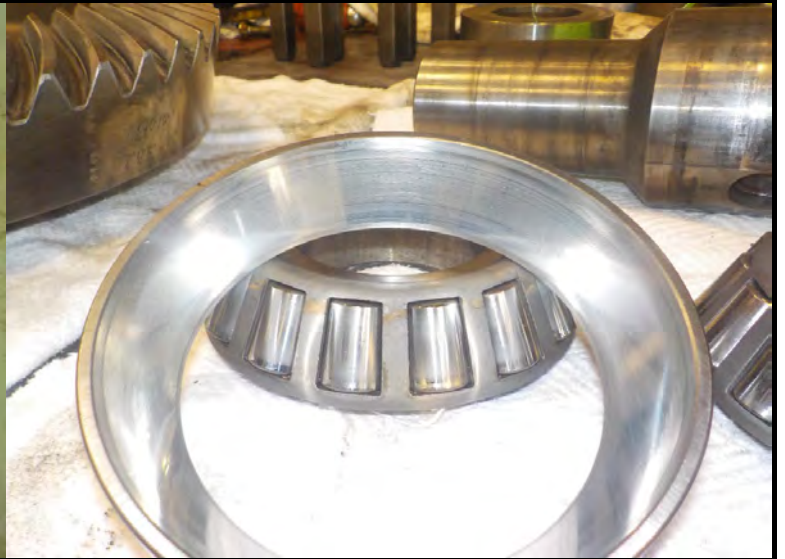
L.S. PINION TAPERED ROLLER BEARING
