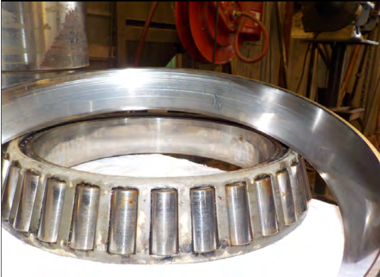
OUTPUT SHAFT TAPERED ROLLER BEARING
