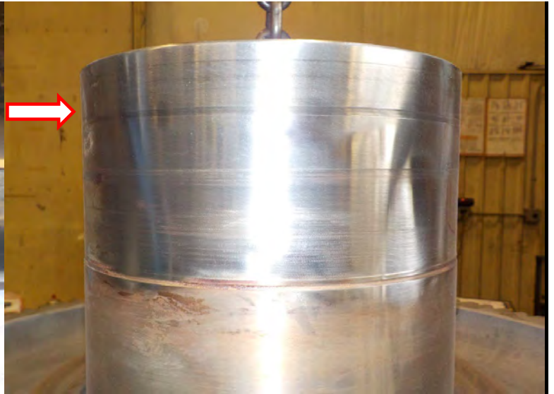
HOLLOW OUTPUT SHAFT SEAL JOURNAL, GROOVED
