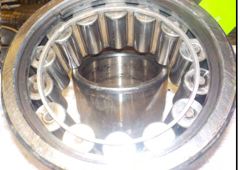
L.S. PINION CYLINDRICAL ROLLER BEARING
