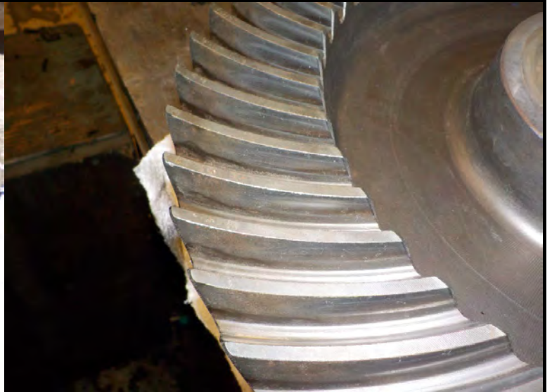
BEVEL GEAR (49T) POLISHING
