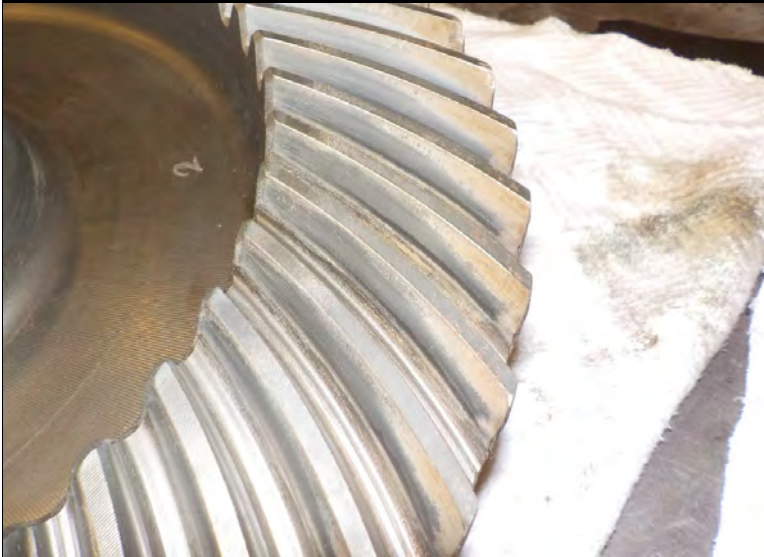
BEVEL GEAR (49T) POLISHING
