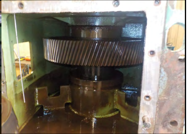
HOUSING CARRIER REMOVED
