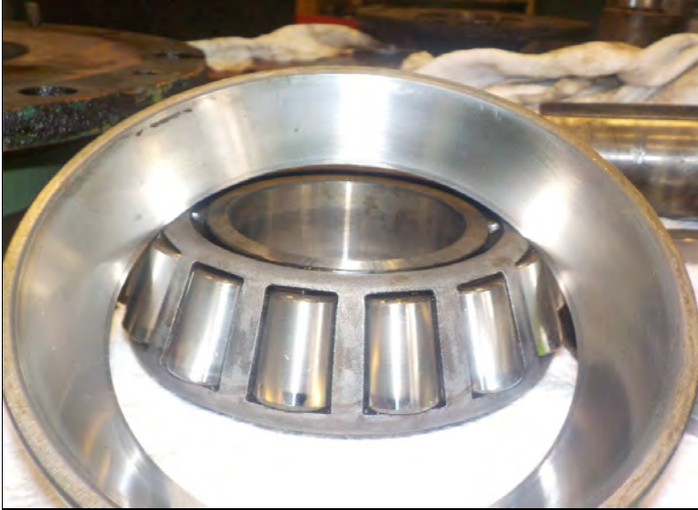
INPUT TAPERED ROLLER BEARING
