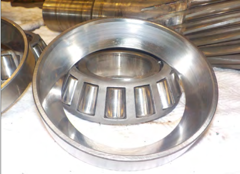
L.S. PINION TAPERED ROLLER BEARING
