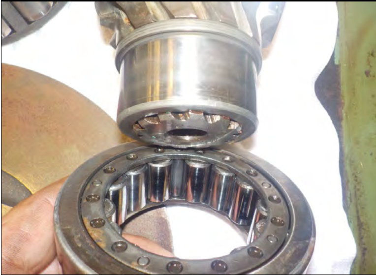
INPUT CYLINDRICAL ROLLER BEARING
