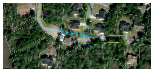
2. Approximately 225 LF of proposed water line loop through Planting Hammock Boulevard connecting the existing 12-inch on South Port Parkway to the existing 8-inch on Callie Circle.
