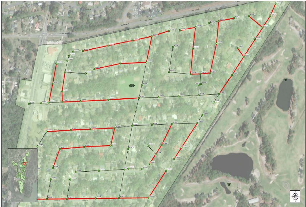
Figure 2 - Map of pipes that indicated leakage
