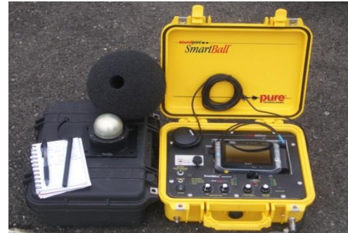
Figure 1: SmartBall Instrument and SmartBall Receiver (SBR)
