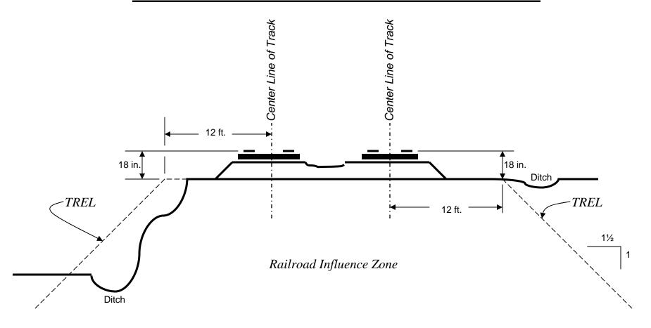
The Theoretical Railroad Embankment Line ("TREL") begins at a point 12 ft. horizontally from center line of track, 18 in. below top-of-rail, and extends downward on a 1½ (H) to 1(V) slope.
