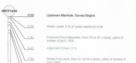
joint: YES Material Change, Concrete pipe (non-reinfored)
