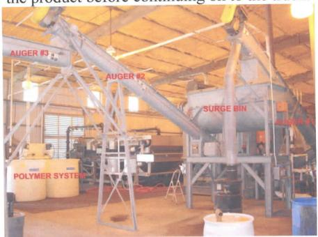
After the product temperature has been brought down auger #2 & #3 take it to the truck to be carried to the mulch facility.
