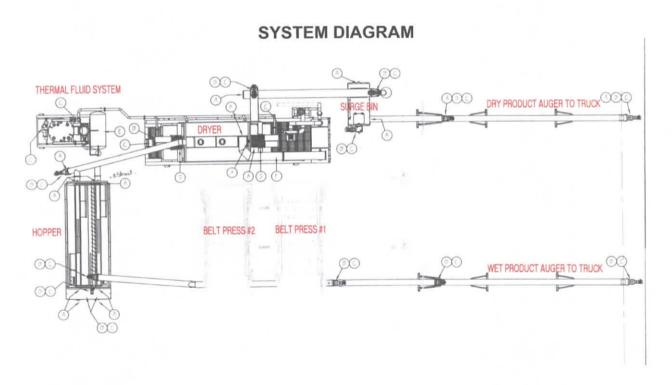
NOTE: If the dryer is down for maintenance, with the turn of a switch the WET PRODUCT AUGER can be turned on and sludge can still be removed to SUPERIOR LANDFILL in Savannah, Georgia.
