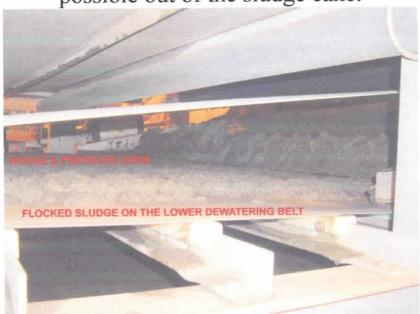
After the sludge cake is ran through the belt press it travels through auger #4 to the hopper.
